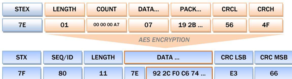
The final complete packet is as follows. The encrypted bytes are highlighted in red.
